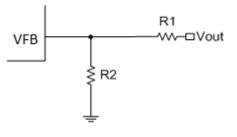
Figure 5 Feedback Divider Network
