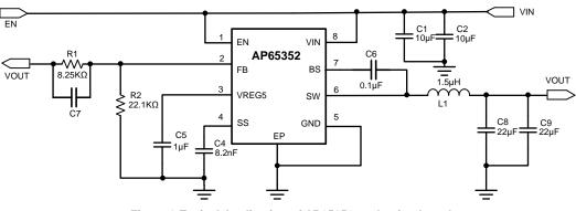
Figure 3 Typical Application of AP65352 evaluation board
