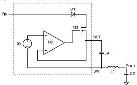
Figure 2—Internal Bootstrap Charging Circuit
