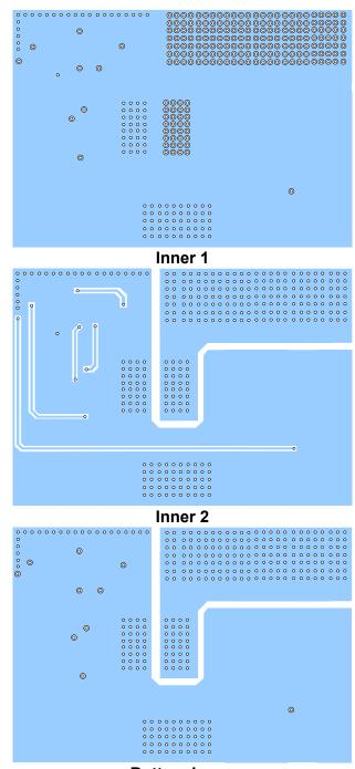
Bottom Layer Figure 4—PCB Layout
