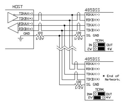
Figure 4. RS-422 Wiring Diagram
