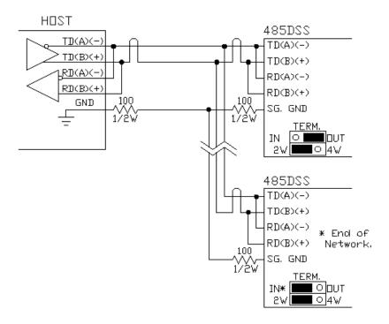
Figure 3. RS-485 Wiring Diagram
