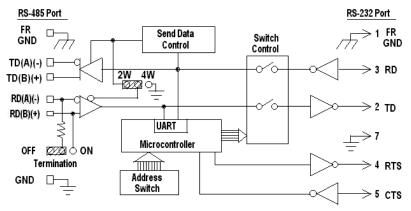
Figure 5. Simplified Functional Diagram
