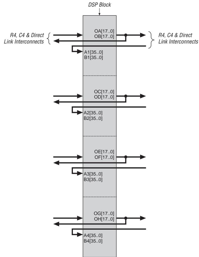
Figure 3-8. Detailed View, DSP Block Interface to Interconnect
