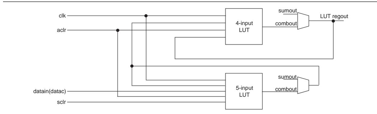
**Figure 2-16.** ALM in LUT-Register Mode with 3-Register Capability
