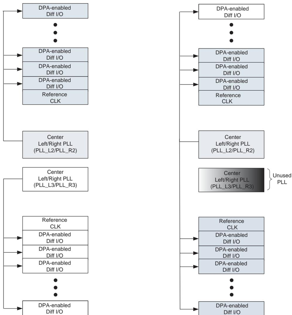
**Figure 9-20.** Invalid Placement of DPA-Enabled Differential I/Os Driven by Both Center Left/Right PLLs
