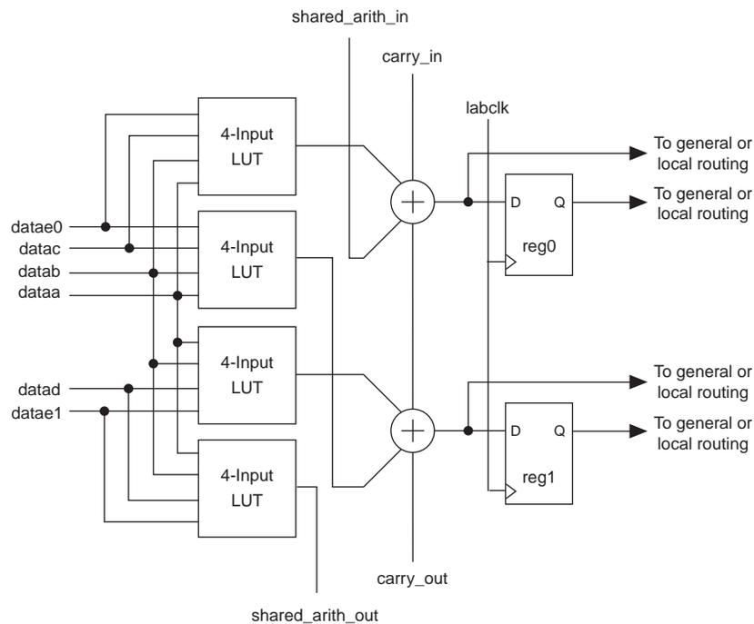
You can find adder trees in many different applications. For example, the summation of the partial products in a logic-based multiplier can be implemented in a tree structure. Another example is a correlator function that can use a large adder tree to sum filtered data samples in a given time frame to recover or to de-spread data that was transmitted utilizing spread spectrum technology.
