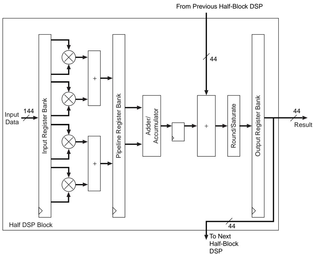
Also shown in [Figure 5-4](#) is the optional Rounding and Saturation Unit (RSU). This unit provides a rich set of commonly found arithmetic round and saturation functions used in signal processing.
