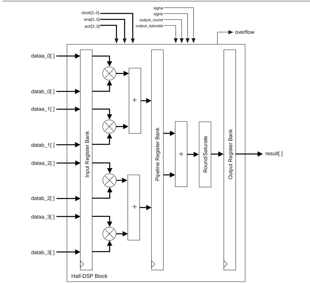
The four-multiplier adder mode supports the round and saturation logic unit. You can use the pipeline registers and output registers within the DSP block to pipeline the multiplier-adder result, increasing the performance of the DSP block.
