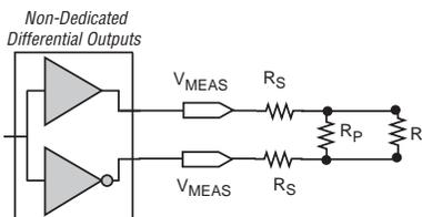
**Table 1-37.** Output Timing Measurement Methodology for Output Pins (Part 1 of 3)
