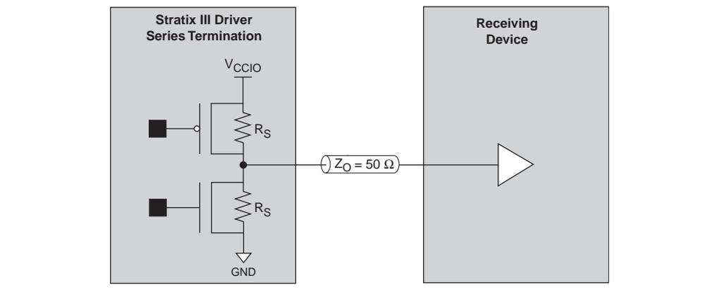
To use OCT for the SSTL Class I standard, you should select the **50-Ω on-chip series termination** setting, eliminating the external 25-Ω  $R_S$  (to match the 50-Ω transmission line). For the SSTL Class II standard, you should select the **25-Ω on-chip series termination** setting (to match the 50-Ω transmission line and the near-end external 50-Ω pull-up to  $V_{TT}$ ).
