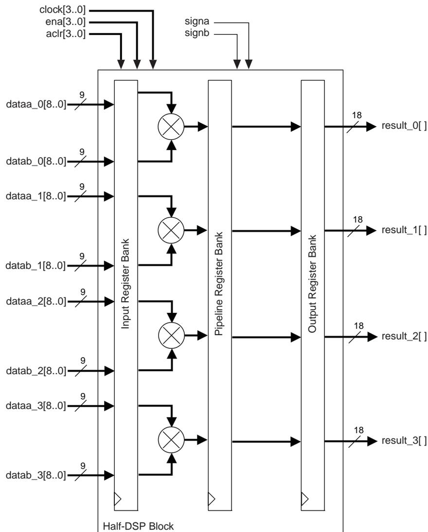
The multiplier operands can accept signed integers, unsigned integers, or a combination of both. You can change the `signa` and `signb` signals dynamically and can be registered in the DSP block. Additionally, the multiplier inputs and result can be registered independently. You can use the pipeline registers within the DSP block to pipeline the multiplier result, increasing the performance of the DSP block.
