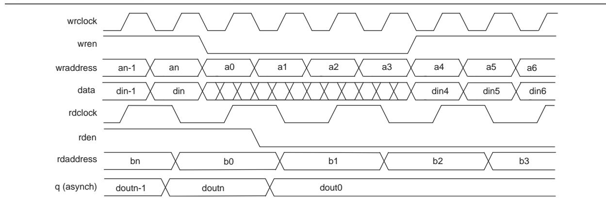
[Figure 4-14](#) shows the timing waveforms for read and write operations in simple dual-port mode with unregistered outputs in MLABs. In MLABs, the write operation is triggered by the falling clock edges.
