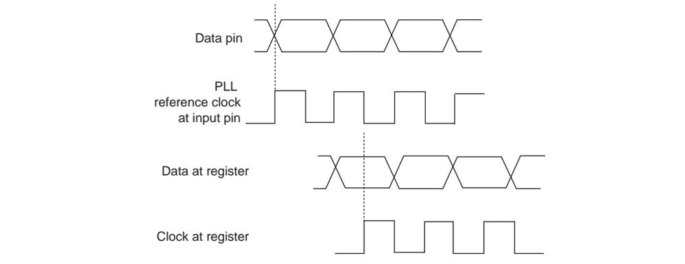
The source-synchronous mode compensates for the delay of the clock network used plus any difference in the delay between these two paths:
