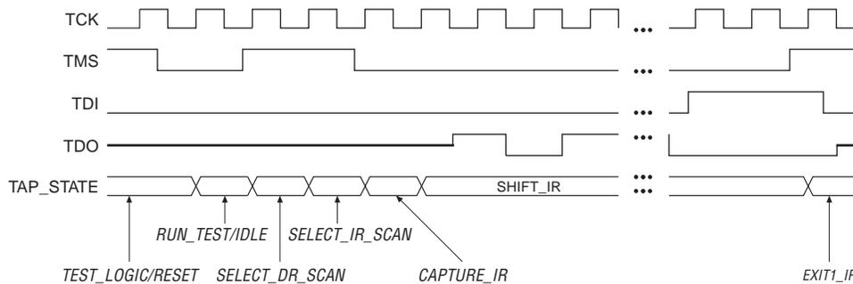
The TDO pin is tri-stated in all states except in the SHIFT\_IR and SHIFT\_DR states. The TDO pin is activated at the first falling edge of TCK after entering either of the shift states and is tri-stated at the first falling edge of TCK after leaving either of the shift states.
