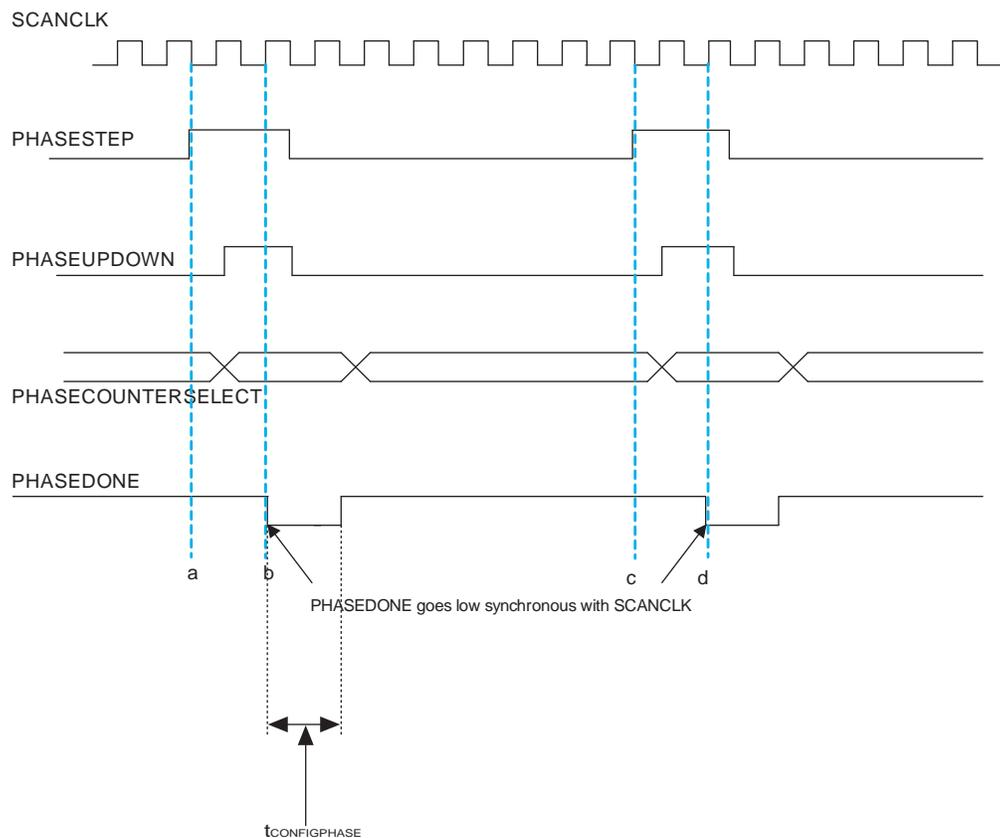
Dynamic phase-shifting can be repeated indefinitely. All signals are synchronous to scanclk and must meet  $t_{su}/t_h$  requirements with respect to scanclk edges.
