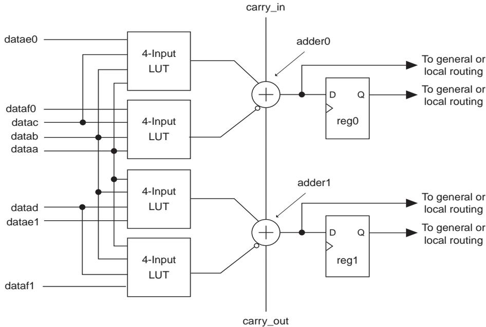
While operating in arithmetic mode, the ALM can support simultaneous use of the adder's carry output along with combinational logic outputs. In this operation, the adder output is ignored. This usage of the adder with the combinational logic output provides resource savings of up to 50% for functions that can use this ability. An example of such functionality is a conditional operation, such as the one shown in [Figure 2-12](#).
