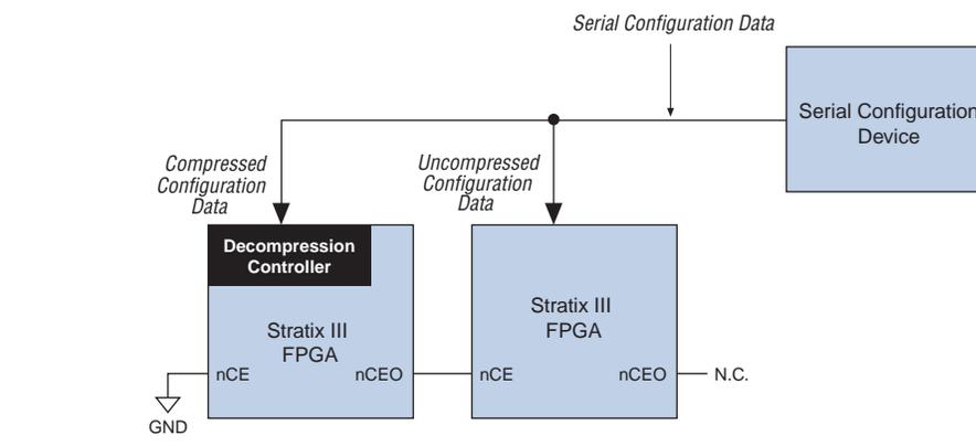
To generate programming files for this setup in the Quartus II software, on the File menu, click **Convert Programming Files**.
