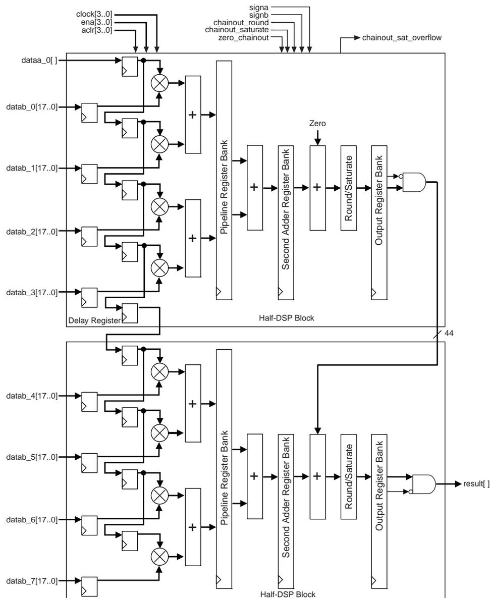
When you use **both** the input cascade and chainout features, the DSP block uses an 18-bit delay register in the boundary of each half-DSP block or from block-to-block to synchronize the input scan chain data with the chainout data. The top half computes the sum of product and chains the output to the next block after the output register. The output register uses the delay register to delay the cascade input by one clock cycle to compensate the latency for the bottom half.
