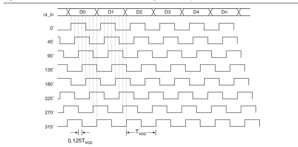
The DPA block continuously monitors the phase of the incoming serial data and selects a new clock phase if required. You can prevent the DPA from selecting a new clock phase by asserting the optional `RX_DPLL_HOLD` port, which is available for each channel.
