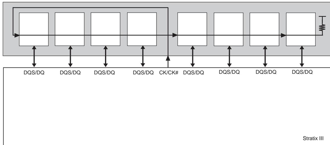
Because the data and read strobe signals are still point-to-point, special consideration must be taken to ensure that the timing relationship between CK/CK# and DQS signals ( $t_{DQSS}$ ) during a write is met at every device on the modules. Furthermore, read data coming back into the FPGA from the memory is also staggered in a similar way.
