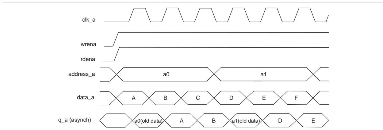
Figure 4-11 shows the timing waveforms for read and write operations in single-port mode with unregistered outputs for MLABs. For MLABs, the read operation is triggered by the rising clock edges whereas the write operation is triggered by the falling clock edges.
