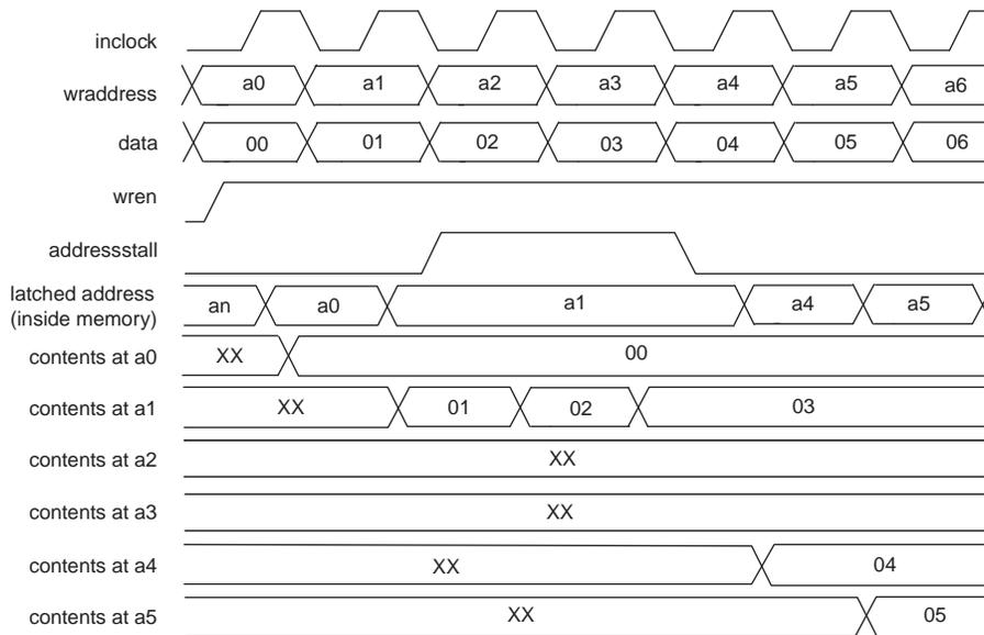
Figure 4-6 shows the address clock enable waveform during the write cycle for MLABs.
