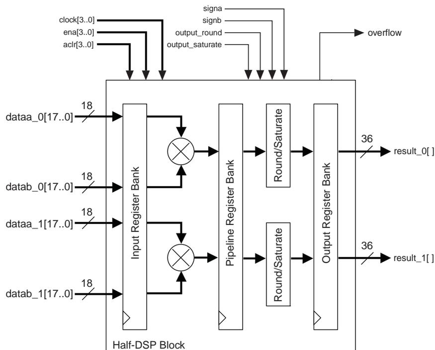
**Figure 5-9.** 12-Bit Independent Multiplier Mode for Half-DSP Block
