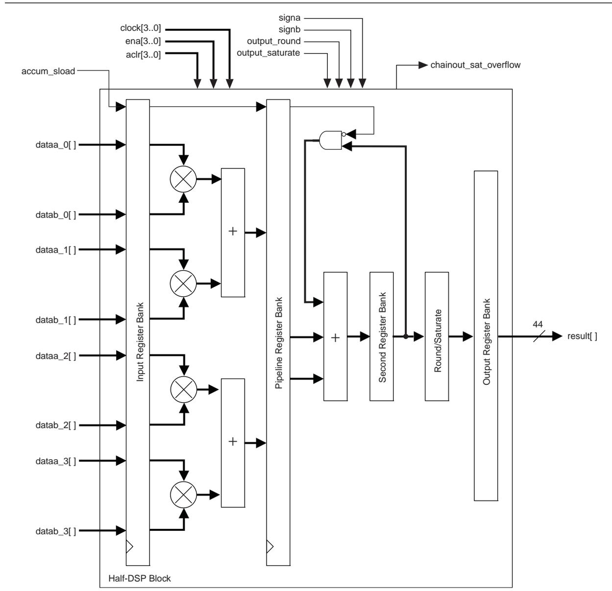
A single DSP block can implement up to two independent 44-bit accumulators.
