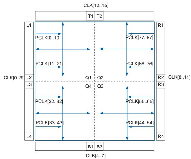
**Figure 6-8.** Peripheral Clock Networks (EP3SE260 Devices)
