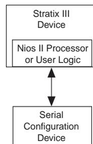
You must set the mode select pins (MSEL[2..0]) to Fast AS mode to use the remote system upgrade in your system. Table 12-1 lists the MSEL pin settings for Stratix III devices in standard configuration mode and remote system upgrade mode. The following sections describe the remote update of remote system upgrade mode.
