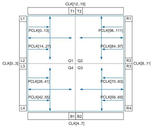
**Figure 6-9.** Peripheral Clock Networks (EP3SL340 Devices)
