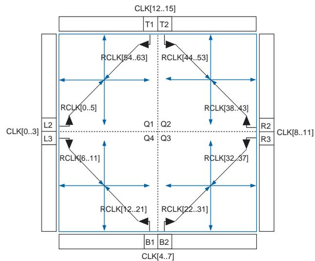
**Figure 6-4.** Regional Clock Networks (EP3SL200, EP3SE260, and EP3SL340 Devices) (Note 1)
