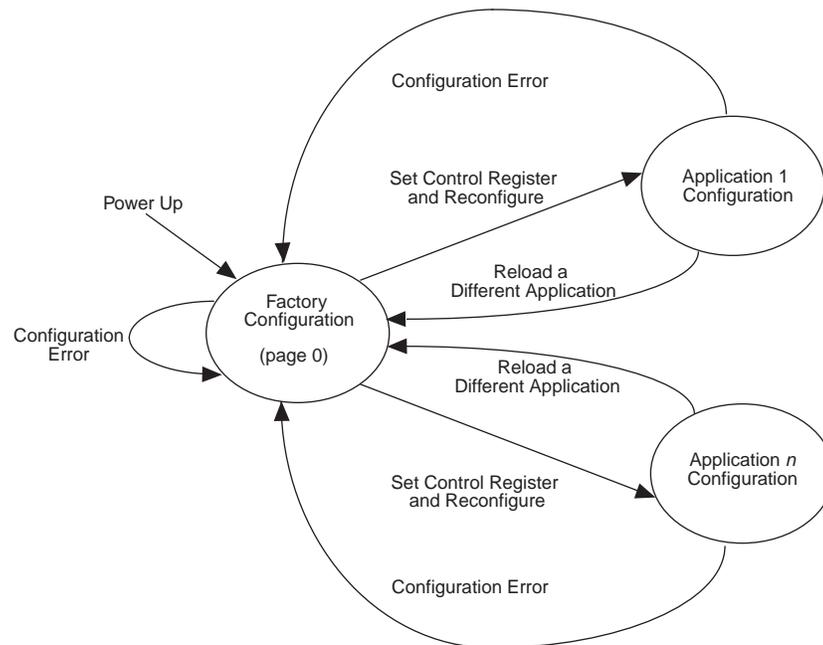
After power up or a configuration error, the factory configuration logic is loaded automatically. The factory configuration also needs to specify whether to enable the user watchdog timer for the application configuration and if enabled, to include the timer setting information as well.
