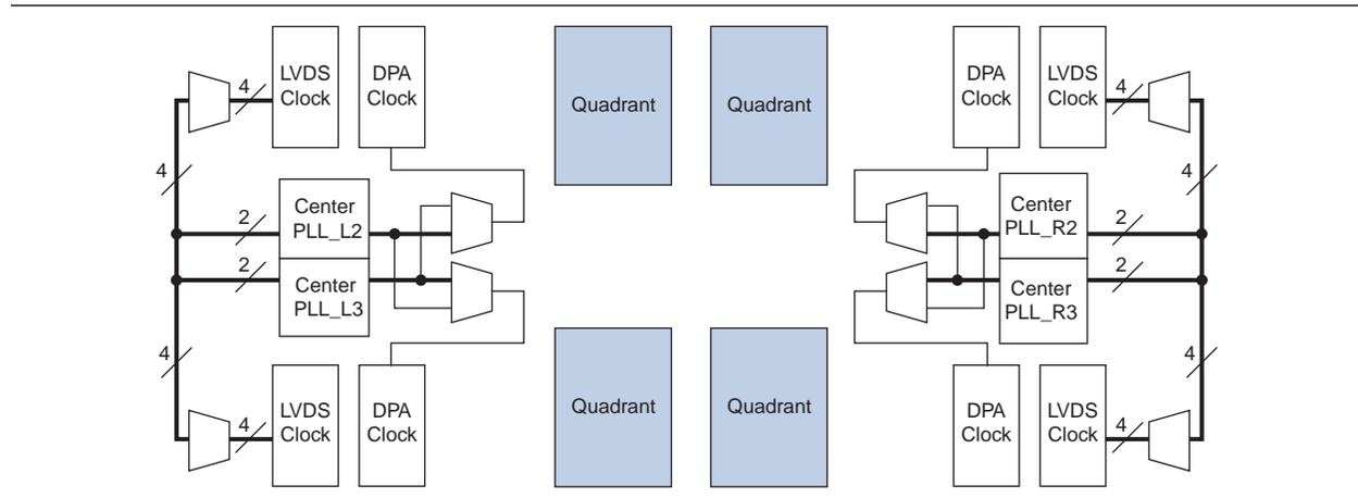
**Figure 9-14.** LVDS/DPA Clocks with Center and Corner PLLs for Stratix III Devices
