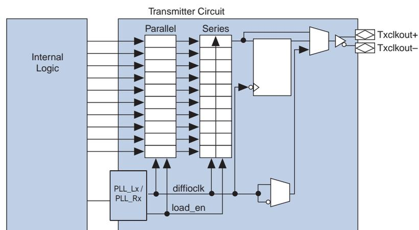
You can bypass the Stratix III serializer to support DDR ( $\times 2$ ) and SDR ( $\times 1$ ) operations to achieve a serialization factor of 2 and 1, respectively. The I/O element (IOE) contains two data output registers that can each operate in either DDR or SDR mode. The clock source for the registers in the IOE can come from any routing resource, from the left/right PLL (PLL\_Lx/PLL\_Rx) or from the top/bottom (PLL\_Tx/PLL\_Bx) PLL.
