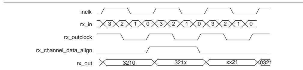
The data realignment circuit can have up to 11 bit-times of insertion before a rollover occurs. The programmable bit rollover point can be from 1 to 11 bit-times, independent of the deserialization factor. An optional status port, `RX_CDA_MAX`, is available to the FPGA from each channel to indicate when the preset rollover point is reached.
