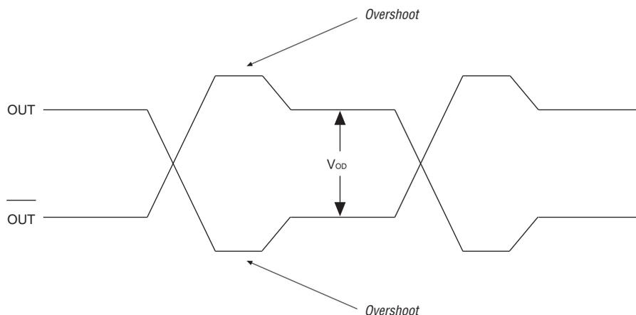
Pre-emphasis is an important feature for high-speed transmission. Without pre-emphasis, the output current is limited by the  $V_{OD}$  setting and the output impedance of the driver. At high frequency, the slew rate may not be fast enough to reach the full  $V_{OD}$  before the next edge, producing a pattern dependent jitter.
