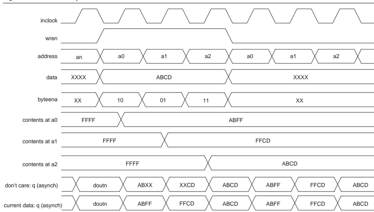
Figure 4-2 shows how the write enable (wren) and byte-enable (byteena) signals control the operations of the MLABs. The write operation in MLABs is triggered by falling clock edges.
