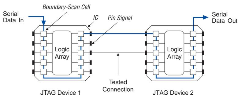
In addition to BST, you can use the IEEE Std. 1149.1 controller for Stratix III device in-circuit reconfiguration (ICR). However, this chapter only discusses the BST feature of the IEEE Std. 1149.1 circuitry.
