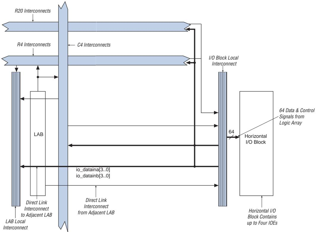
Figure 3-10. Column I/O Block Connection to Interconnect
