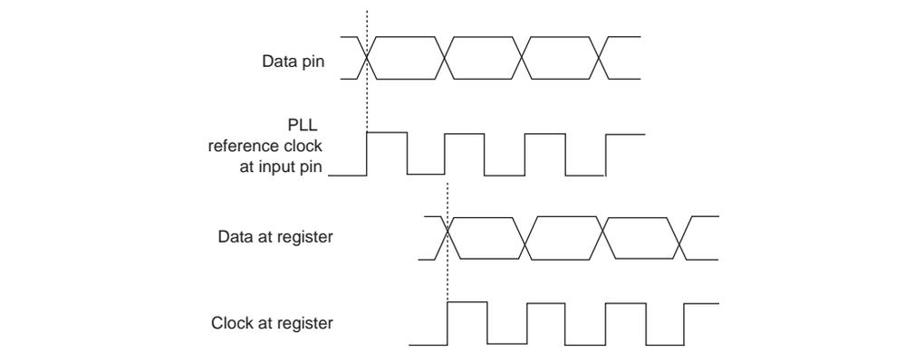
**Figure 6-24** shows an example waveform of the clock and data in the LVDS mode.
