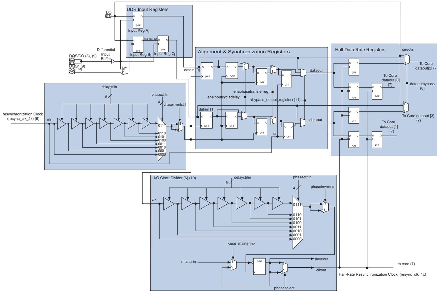
**Figure 8–20.** Stratix III IOE Input Registers (Note 1)**Notes to Figure 8–20:**
