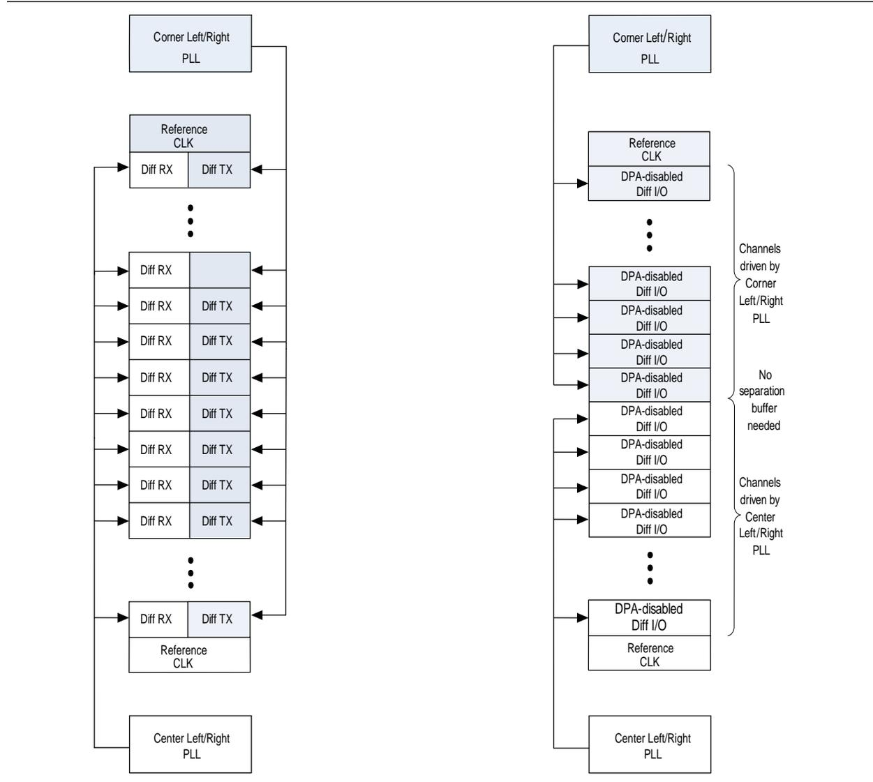
**Figure 9-22.** Invalid Placement of DPA-Disabled Differential I/Os Due to Interleaving of Channels Driven by the Corner and Center Left/Right PLLs
