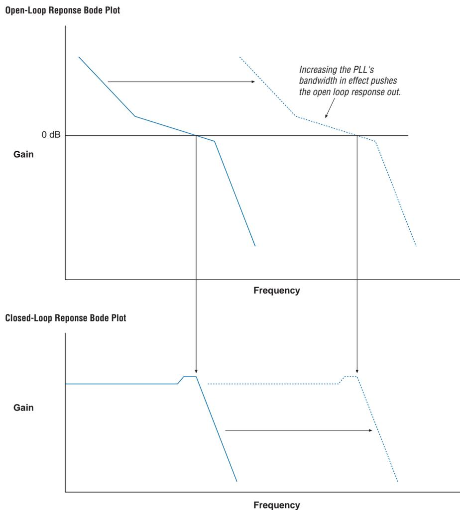
A high-bandwidth PLL provides a fast lock time and tracks jitter on the reference clock source, passing it through to the PLL output. A low-bandwidth PLL filters out reference clock jitter but increases lock time. Stratix III PLLs allow you to control the bandwidth over a finite range to customize the PLL characteristics for a particular application. The programmable bandwidth feature in Stratix III PLLs benefits applications requiring clock switchover.
