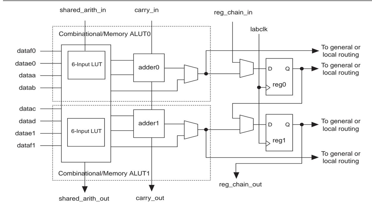
Each ALM has two sets of outputs that drive the local, row, and column routing resources. The LUT, adder, or register output can drive these output drivers (refer to [Figure 2-6](#)). For each set of output drivers, two ALM outputs can drive column, row, or direct link routing connections, and one of these ALM outputs can also drive local interconnect resources. This allows the LUT or adder to drive one output while the register drives another output.
