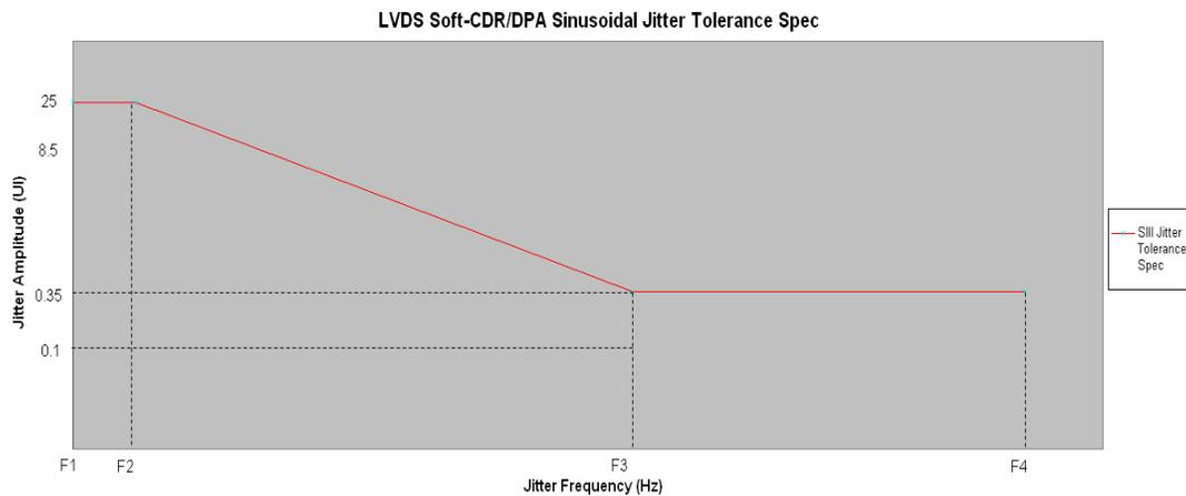
Table 1-27 lists the LVDS Soft-CDR/ DPA sinusoidal jitter mask values for Stratix III devices.
