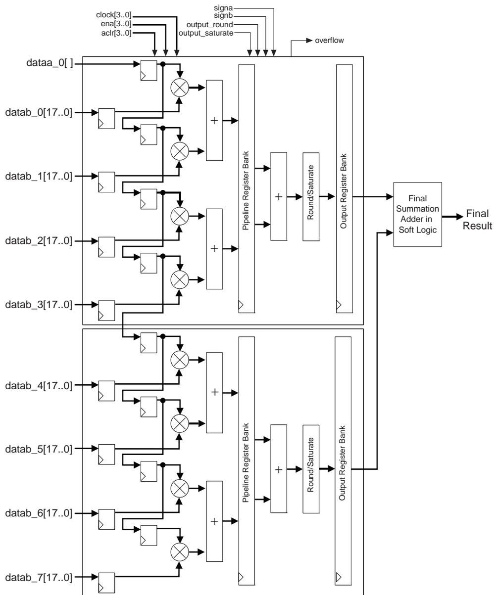
For faster and more efficient chained cascade summation, the DSP block can implement the chainout function in the cascade mode. This mode uses the second-stage 44-bit adder to add the current Four-Multiplier Adder of the half DSP block to the adjacent half DSP block of the Four-Multiplier Adder as shown in [Figure 5-23](#).
