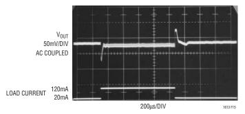
Figure 15. 5V Output SEPIC with  $10\mu F$  Ceramic Output Capacitor, 330pF  $C_{PL}$  and 10k in Series with FB Pin
