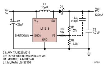
Figure 10. 5V to 12V Boost Converter with 4.7 $\mu$ F Ceramic Output Capacitor, C<sub>PL</sub> Added to Increase Phase Margin
