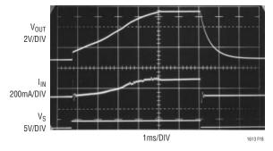
Figure 19. Increasing C<sub>S</sub> to 33nF Further Reduces Inrush Current.  $R_{LOAD} = 50\Omega$
