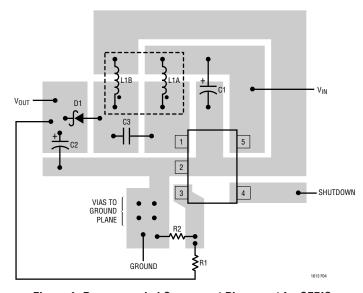
Figure 4. Recommended Component Placement for SEPIC
