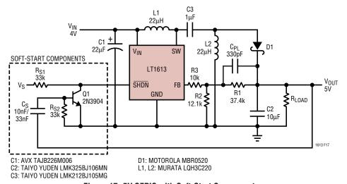
Figure 17. 5V SEPIC with Soft-Start Components
