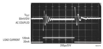
Figure 14. 5V Output SEPIC with  $10\mu F$  Ceramic Output Capacitor. No  $C_{PL}$ .  $V_{IN}=4V$
