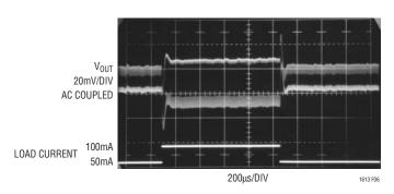
Figure 6. 2.5V to 5V Boost Converter Transient Response with 22 $\mu$ F Tantalum Output Capacitor. Apparent Double Trace on V<sub>OUT</sub> Is Due to Switching Frequency Ripple Current Across Capacitor ESR
