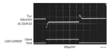
Figure 12. 5V to 12V Boost Converter with 4.7  $\mu\text{F}$  Ceramic Output Capacitor and 200pF Phase-Lead Capacitor C<sub>PL</sub> and 10k in Series with FB Pin
