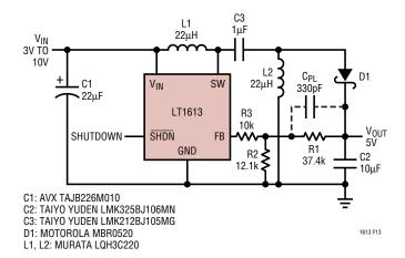
Figure 13. 5V Output SEPIC with Ceramic Output Capacitor. C<sub>PL</sub> Adds Phase Margin
