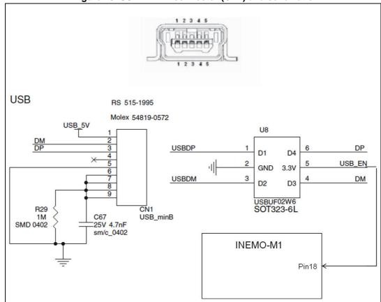
Figure 10. USB mini-B connector (CN1) and schematic
