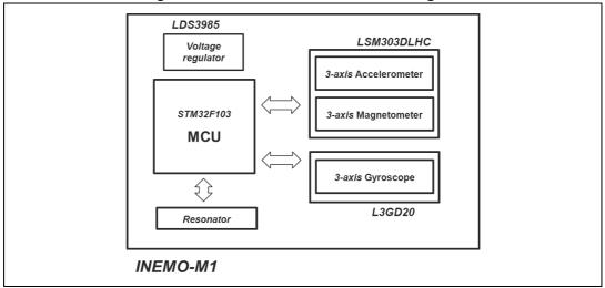
Figure 7. INEMO-M1 functional block diagram
