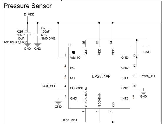
Figure 25. Pressure sensor
