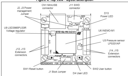
Figure 4. Top view - layout description
