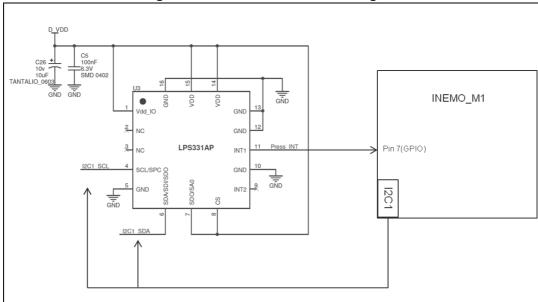
Figure 8. Pressure sensor block diagram
