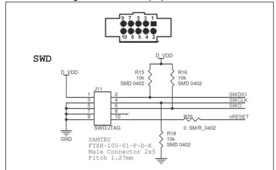
Figure 9. SWD connector (J11) and schematic
