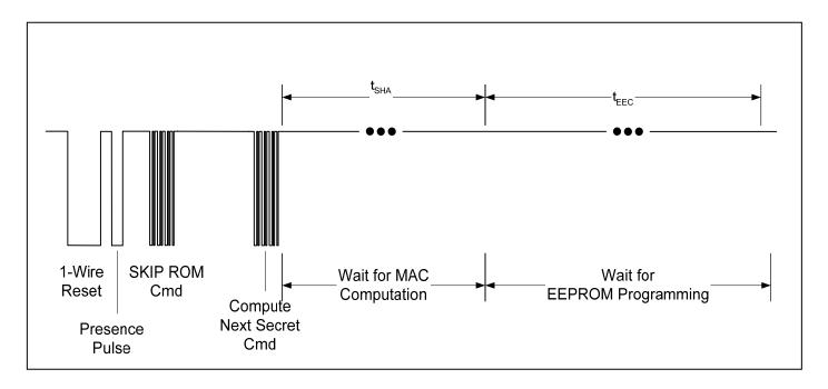
Figure 9. Copy Scratchpad Function Command
