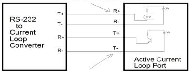
Note: The T+ & T- indentification doesn't imply a direct connection across the transmitter.
