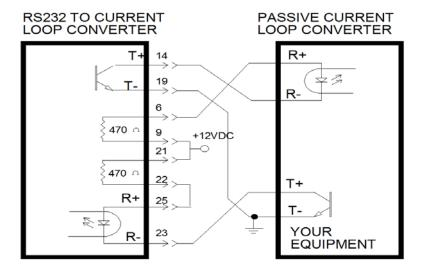
Figure 3. Connection to a Passive Current Loop
