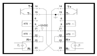
Figure 4. Interconnection of Two Current Loop converters
