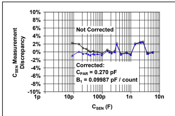
**FIGURE 9:**  $C_{SEN}$  Measurement Discrepancy.
