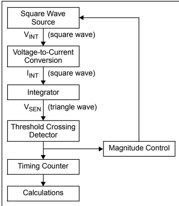
**FIGURE 1:** Integrator Block Diagram.
