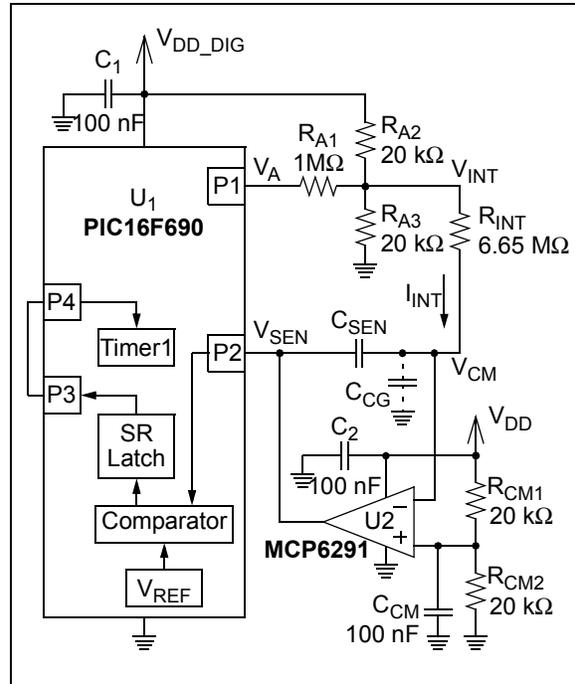
**FIGURE 6:** Op Amp Integrator Circuit with Reduced Current.
