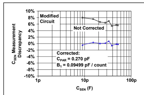
**FIGURE 8:**  $C_{SEN}$  Measurement Discrepancy.
