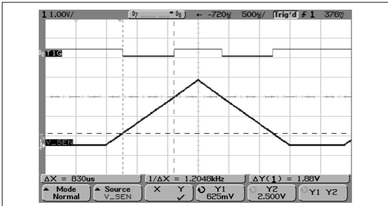
**FIGURE 7:**  $V_{INT}$  and  $V_{SEN}$  Waveforms with  $C_{SEN} = 166$  pF.
