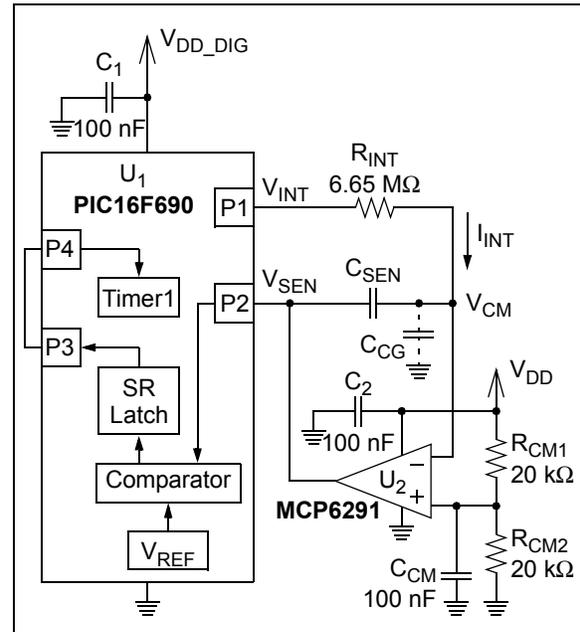
**FIGURE 3:** Op Amp Integrator Circuit.
